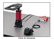
[APPLIST] MCM301 Controller and MCMK3 Three-Knob Joystick Used to Control Both Axes of the PLSXY Translation Stage and One-Axis MPM250 Motorized Rigid Stand
