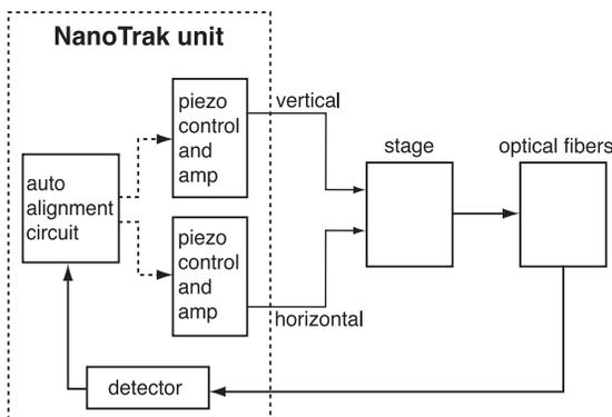
Block Diagram: With one fiber fixed and the other mounted on a piezo-actuated stage capable of moving the fiber perpendicular to its end face, the NanoTrak™ controls the position of the moving fiber. The NanoTrak’s auto-alignment circuit controls the position of the fiber as it optimizes the efficiency of the butt-coupling. In many applications, a planar waveguide or other device replaces one of the fibers; however, the basic principles remain the same.
