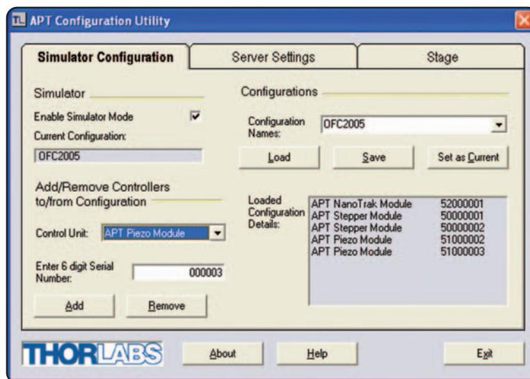
It also gives the option of developing custom applications off-line if, for example, the apt™ hardware is unavailable or already being used. Moreover, after an apt™-based custom application has been developed and released, the actual physical apt™ hardware may no longer be accessible for software support and maintenance purposes, and so a simulator mode proves invaluable.
