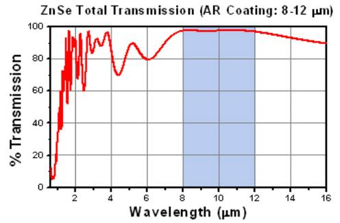
Shown above is a graph of the theoretical transmission of the AR-coated zinc selenide plano-convex lens. The blue shaded region denotes the 8 - 12 µm spectral range where the AR coating is optimized. For this wavelength range, the measured transmission is in excess of 97%.
