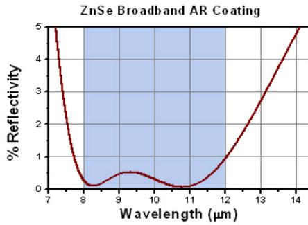
Shown above is a theoretical graph of the percent reflectivity of the AR coating as a function of wavelength. The average reflectivity in the 8 - 12 µm range is <1.5%. The blue shading indicates the region for which the AR coating is optimized.
