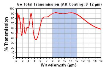
Shown above is a graph of the theoretical transmission of the AR-coated germanium plano-convex lens. The blue shaded region denotes the 8 - 12 µm spectral range where we suggest using these Ge plano-convex lenses. For this wavelength range, the measured transmission is in excess of 88%.
