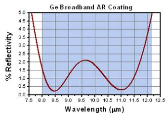
Shown above is a theoretical graph of the percent reflectivity of the AR coating as a function of wavelength. The average reflectivity in the 8 - 12 µm range is <1.5%. The blue shading indicates the recommended usage range for these Ge plano-convex lenses.
