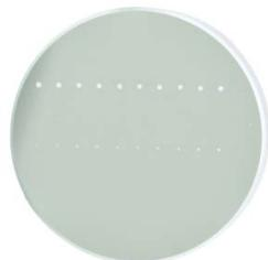
The photograph above is a protected aluminum-coated mirror after LIDT testing. In this particular test, it handled 0.43 J/cm<sup>2</sup> (1064 nm, 10 ns pulse, 10 Hz, Ø1.000 mm) before damage.
