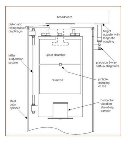
This restriction of airflow damps oscillatory motion between the floor and breadboard, dramatically reducing settling time. The volume ratio of the chambers has been optimized to maximize damping performance for our complete range of breadboards while preserving a low resonant frequency.
