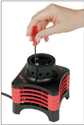
Figure 1: Remove the two screws holding the lens tube in place using a 2.5 mm hex key or balldriver.
