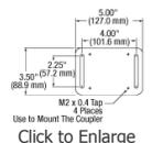
Our FCQB mounting base provides two 2.25" (57.2 mm) long clearance slots for 1/4" (M6) cap screws for mounting Thorlabs' RGB wavelength combiners or 1x4 couplers to an optical table or other tapped surface. The two clearance slots are located 4" (101.6 mm) apart at opposite edges of the mounting base. Four M2 taps between the clearance slots are positioned to align with the through holes in Thorlabs' RGB wavelength combiners and 1x4 SM couplers. Four M2 screws are included.
