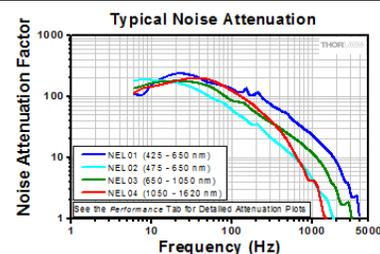
Noise Attenuation Factor is the Ratio of Noise Amplitude Before and After the Noise Eater
