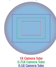
As the magnification increases, the resolution improves, but the field of view also decreases. The dependence of the field of view on magnification is shown in the schematic to the right.
