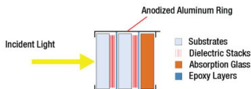
The number of layers shown in this schematic is not indicative of the number of layers in an actual bandpass filter. Also the drawing is not to scale.
