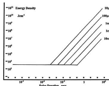
LIDT in energy density vs. pulse length and spot size. For short pulses,
