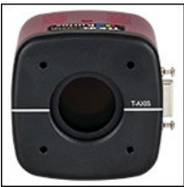
Click to Enlarge The front of the filter head contains internal SM1 or SM2 threads, four 4-40 taps for cage systems, and an engraving for the transmission axis.
