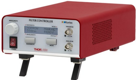
Click to Enlarge The front panel of the KURIOS-WB1/M controller while it is set to manual mode.
