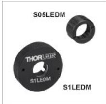
The S05LEDM and S1LEDM LED Mounts are SM05 (0.535"-40) and SM1 (1.035"-40) threaded, respectively. They are designed to hold any of Thorlabs' TO-18, TO-39, TO-46, or T1-3/4 packages using the included adapter rings. The external threading on these mounts allows them to be used in a wide variety of SM05- or SM1-
