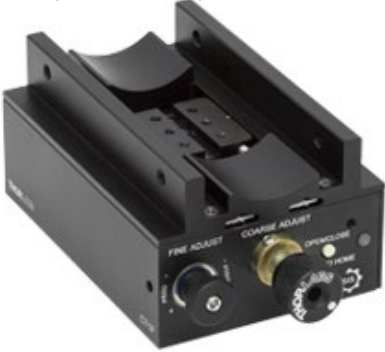
CT1P 12 mm Travel with M6 x 0.25 Screw, 160 \mu m Closed-Loop Piezo Travel
