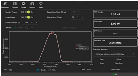
Click to Enlarge Figure 5.1 Bypass Mode allows the user to turn on the amplifier and provides information about the amplified 1035 nm output. Readouts are included for the 1030 energy and power, as well as the repetition rate. The 1030 spectrometer displays the live spectrum of the pulse being sent to the 1035 nm amplifier (white), as well as a reference spectrum (red).
