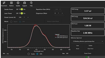
Click to Enlarge Figure 5.2 OPA Mode allows the user to turn on the amplifier and provides information about the 1650 nm OPA power and energy. Readouts are included for the 1030 energy and power, OPA power, and repetition rate. The OPA spectrometer displays the live spectrum of the second harmonic of the OPA output as a proxy for the 1650 nm signal (white), as well as a reference spectrum (red).
