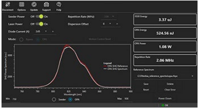
Click to Enlarge Figure 1.2 The FSLOPAX1 software provides a simple GUI to control the laser while providing system feedback. The GUI allows the user to select the laser mode, which either routes the 1035 nm light directly out of the box (Bypass mode) or through the OPA (OPA mode).
