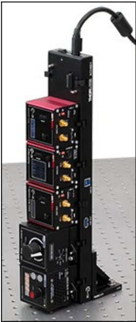
Click to Enlarge [APPLIST] [APPLIST] Figure 1.2 The controller hubs contain M6 taps on the bottom, allowing them to be mounted vertically using the AP90(/M) Right Angle Bracket (sold separately).
