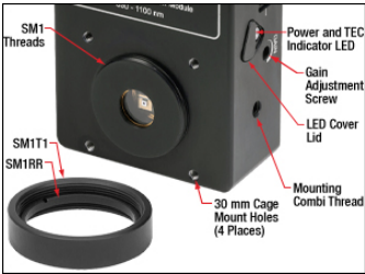
Click to Enlarge Figure G1.1 The SPDMA detection module has external SM1 threads, is 30 mm cage system compatible, and includes an SM1T1 Internal SM1 Adapter and SM1RR Retaining Ring. The module also includes a gain adjustment screw and status LED with cover.
