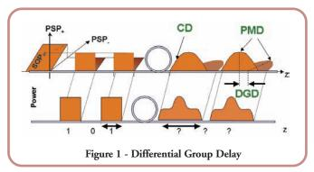
DGD is the primary measurement parameter for all PMD meters. The measurement of the DGD involves the determination of a phase change (arrival time difference) for a given frequency (wavelength) change. For a Jones Matrix Eigenanalysis, the polarization transformation function (the Jones Matrix) must be determined at two different wavelengths. The changes in the phases of the two Jones matrices divided by the wavelength difference (step size) yields the DGD value.
