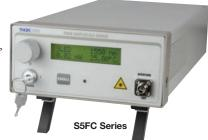
The system's microcontroller actively regulates the drive current and temperature of the SLD as well as monitors the system for fault conditions. The microcontroller has a USB interface that allows for remote adjustment of the output power and temperature of the SLD as well as the enabling of the SLD output.
