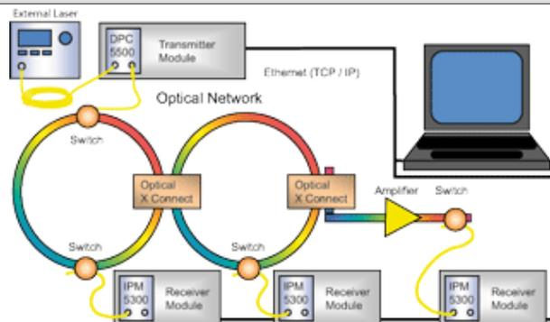
**PMD and PDL Analysis System for a Live Fiber with Traffic
