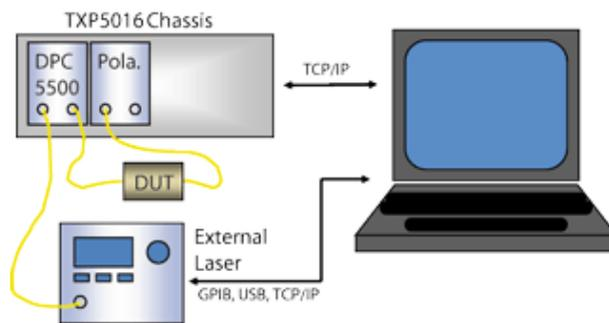
**PMD and PDL Analysis System for Optical Networks
