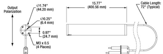
Note that the output polarization applies only to lasers linearly polarized.
