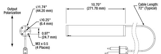
Thorlabs' cylindrical, 2.0 mW, red (632.8 nm) Helium-Neon lasers feature a tube design that makes them easy to mount in nearly any optical system. These lasers are
