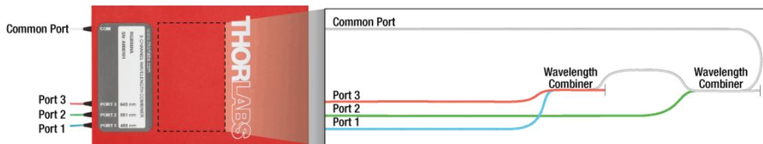
Schematic of the internal components of an example RGB Combiner. The zoom panel shows an example configuration of how (ports 1 - 3) are combined into the common port.
