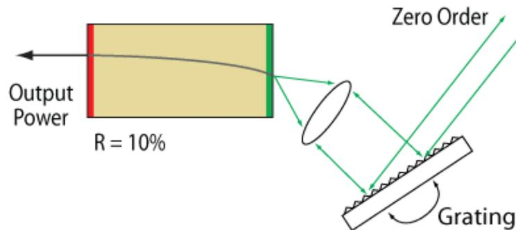
**Figure 5:** Littrow External Cavity Laser
