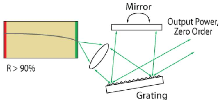
**Figure 6:** Littman-Metcalf External Cavity Laser
