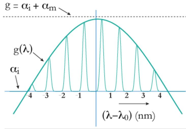
**Figure 2:** Gain Curve of a Fabry-Perot Laser
