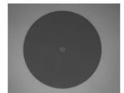
[Click to Enlarge Undamaged Fiber End](#)
