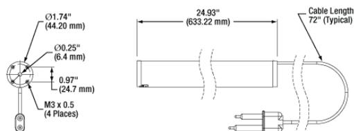
Thorlabs' cylindrical, 15.0 mW, red (632.8 nm) Helium-Neon lasers feature a tube design that makes them easy to mount in nearly any optical system. These lasers are offered with random polarization. A built-in interlock circuit is included that can be integrated with lab safety systems (see *Interlock Disassembly* tab for details). These randomly polarized lasers include external power supplies in 120 VAC, 230 VAC, or 100 VAC versions for compatibility with international power sources.
