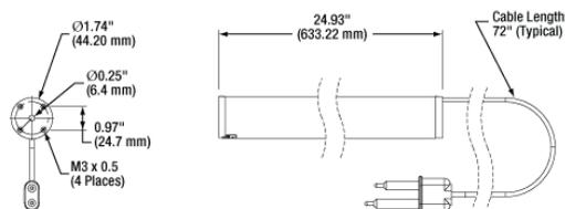
Thorlabs' cylindrical red (632.8 nm) Helium-Neon lasers feature a tube design that makes them easy to mount in nearly any optical system. The HNL225R model offers a 22.5 mW, randomly polarized output. A built-in interlock circuit can be integrated with lab safety systems (see *Interlock Disassembly* tab for details). The included external power supply is compatible with 120 VAC.
