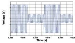
**Figure B.** A plot of the output voltage of the LCC25 Liquid Crystal Controller when the output voltage is being modulated between the two set voltages.
