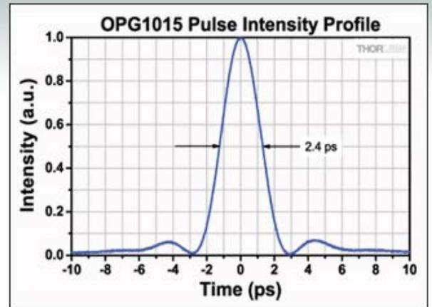
A Typical Pulse From the OPG1015. The UTM-1500 Temporal Magnifier Expands the Pulse for Analysis with a Fast Photodiode and Sampling Oscilloscope
