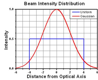
The calculation above assumes a uniform beam intensity profile. You must now consider hotspots in the beam or other non-uniform intensity profiles and roughly calculate a maximum power density. For reference, a Gaussian beam typically has a maximum power density that is twice that of the uniform beam (see lower right).
