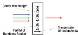
Several filters below are designed for gas absorption lines at 2.30  $\mu\text{m}$  (CO), 3.33  $\mu\text{m}$  (CH<sub>4</sub>), 4.26  $\mu\text{m}$  (CO<sub>2</sub>), 5.068  $\mu\text{m}$  (H<sub>2</sub>O), or 5.33  $\mu\text{m}$  (NO). These filters have narrower transmission bands and sharper transmission peaks. The green highlighted rows in the tables below denote narrowband filters for gas absorption lines.
