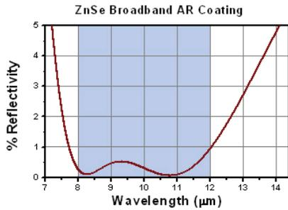
Shown above is a graph of the theoretical percent reflectivity of the AR coating as a function of wavelength. The average reflectivity in the 8 - 12 µm range is <1.5%. The blue shading indicates the region for which the AR coating is optimized.
