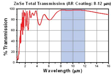
Shown above is a graph of the theoretical transmission of the AR-coated zinc selenide Bi-Convex lens. The blue shaded region denotes the 8 - 12 µm spectral range where the AR coating is optimized. For this wavelength range, the measured transmission is in excess of 97%.
