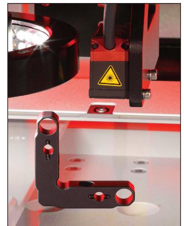
Laser Probe Being Used to Measure Surface Flatness
