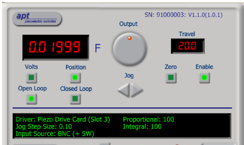
Fig. 4.7 GUI Display - Force Sensor Mode
