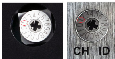
Fig. 4.2 ID switch settings
