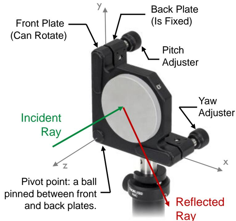
**Figure 10.** Mirror mounted in a KM200 kinematic mirror mount.
