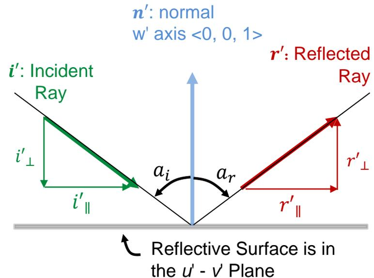
**Figure 3.** The angle between the incident ray and surface normal equals the angle between the reflected ray and surface normal.
