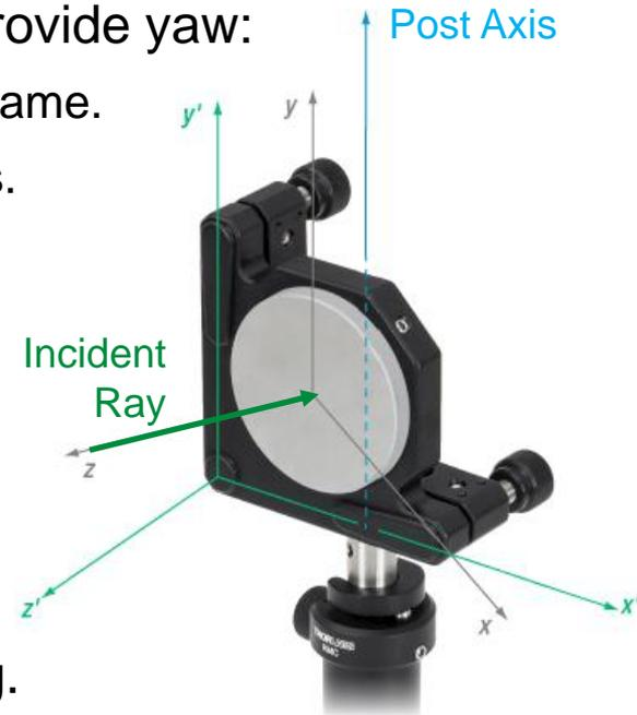
Figure 16. Rotation Axes
