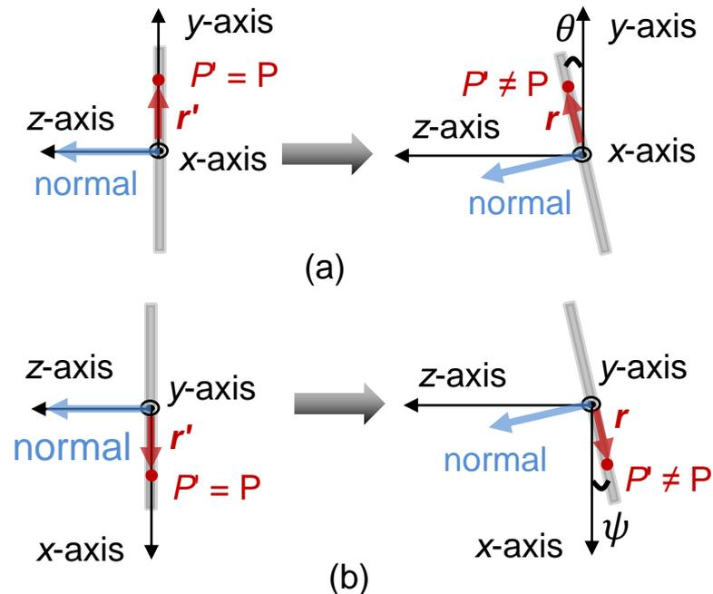
**Figure 7.** Rotation around the (a) x-axis and (b) y-axis. Unrotated surface is on the left, rotated surface is on the right.
