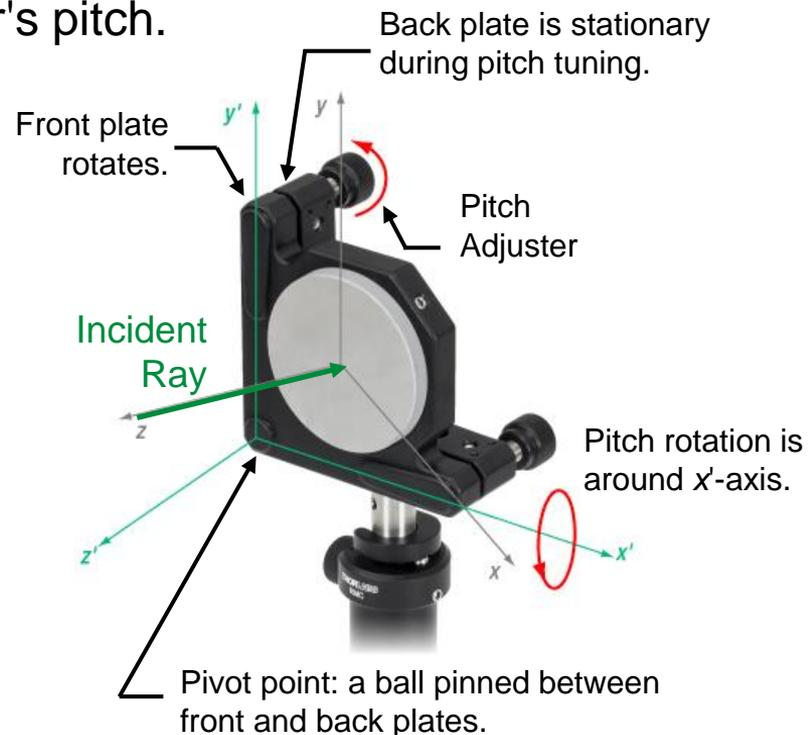
**Figure 15.** Mirror mounted in a KM200 kinematic mirror mount.
