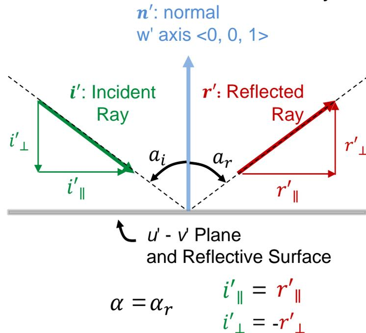
**Figure 12.** Reflection is performed using local coordinates, which involves reflecting the incident ray across the normal to the  $u$ - $v$  plane.
