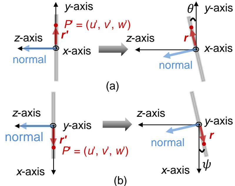
**Figure 8.** Counterclockwise (CCW) rotation around the (a) x-axis and (b) y-axis. Unrotated surface is on the left, rotated surface is on the right.
