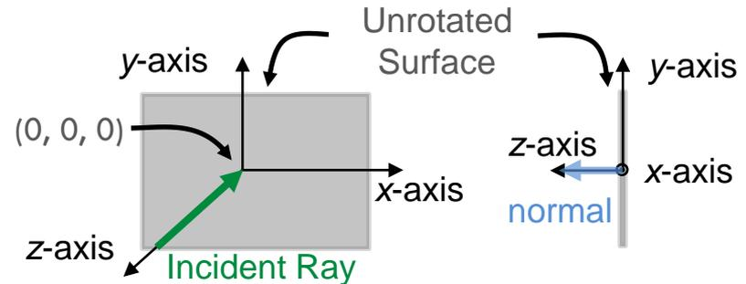
**Figure 5.** First step to a global view is defining the orientation of the unrotated surface.
