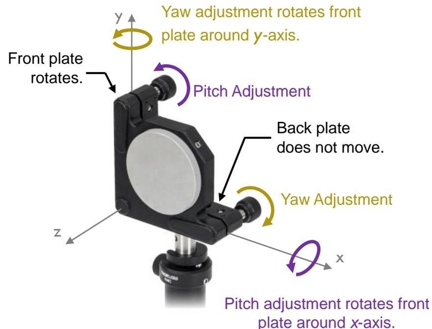
**Figure 11.** Adjusters can be used to tune the mirror's pitch and yaw.
