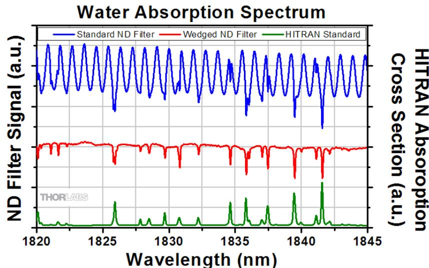
Spectra of water absorption lines using standard (blue) and wedged (red) ND filters compared to the HITRAN spectrum of water (green). Spectra offset and plotted in arbitrary units to visualize differences. It is important to note that this result describes a brief investigation to provide insights into the general behavior of our components and should be interpreted with the specified limitations of the devices in mind.
