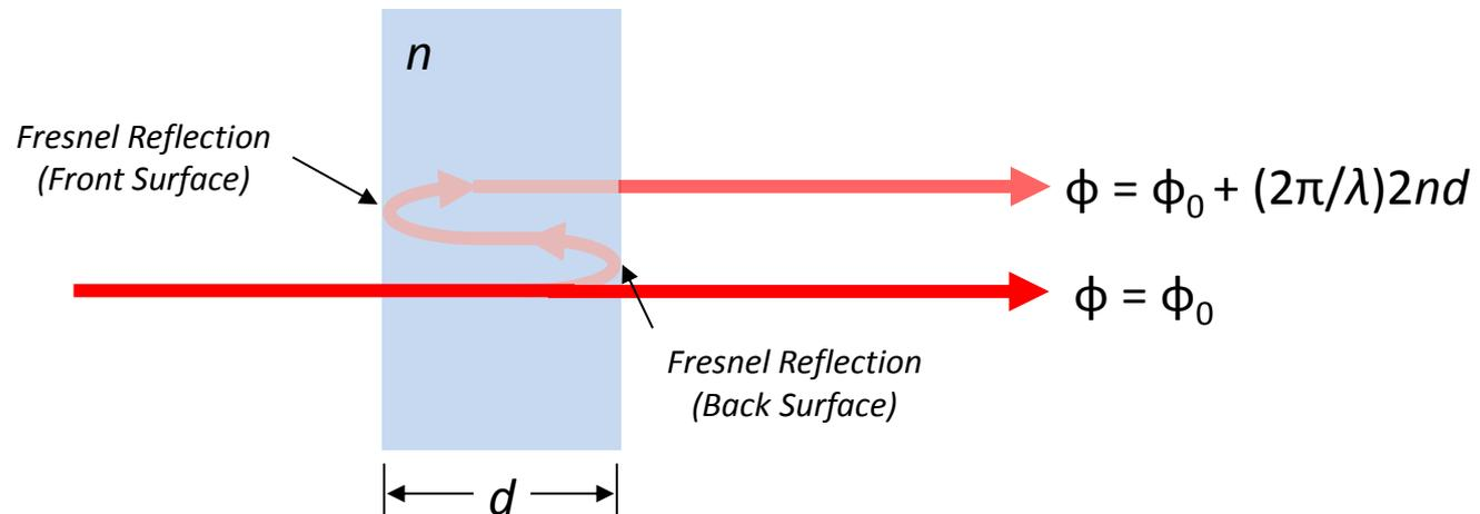
The above is an illustration of Fresnel reflections in a substrate with an index of refraction of  $n$ . The displacement of the beam path shown above is for pictorial clarity and does not represent the actual beam path, which would be coaxial at normal incidence
