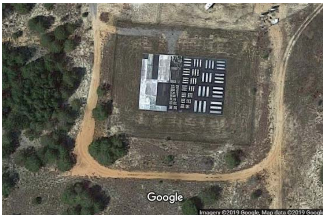
Figure 1: An eye chart for satellites: this huge (50 meter) resolution target, used for testing satellite and aircraft surveillance cameras, is laid out on the ground at Eglin Air Force Base in Florida. If you blow the image up (magnify it) on your computer, can you tell the bars apart in the smallest 3-bar sets on the left in the image? Is more magnification helping, or do you really need better resolution ? (Image Source: https://goo.gl/maps/4L6hPbFamM72 - also available under the Reference Links tab at www.thorlabs.com/OMC )
