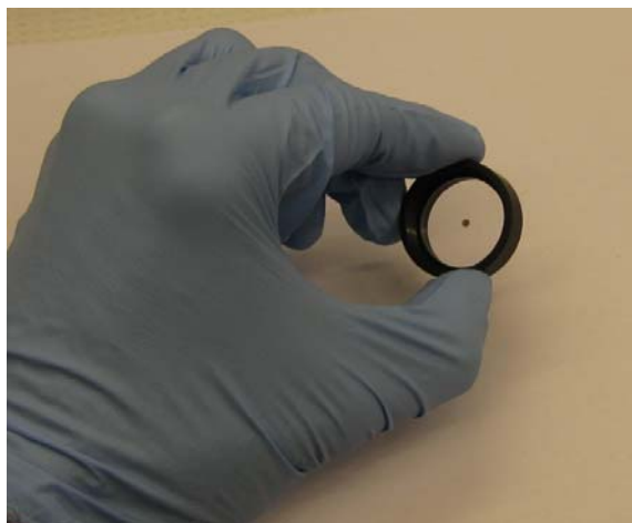
Figure 1: Home-Made Phase Mask: 1.25 mm diameter stearin candle soot spot, with transmission \sim 10\% , on a coverslip mounted in an SM1 tube.
