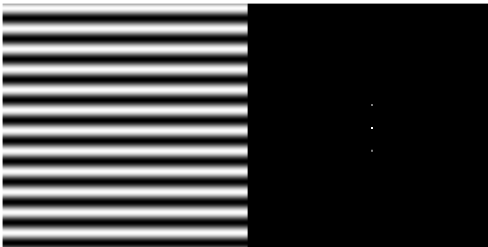
Figure 17: Horizontal sine wave: f(y) = \frac{1}{2} [1 + \sin(2\pi k y)] Diffraction pattern is three dots, as discussed above and in Fig. 9
