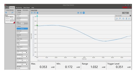
When using the mode SCOPE, additional settings appear in the settings panel and the display panel:
