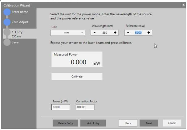
When the calibration is done the following screen appears. To ensure that the calibration is within a reasonable range, the calibration is limited to values differing less that 20% from the reference values. An error message appears if the sensor that is calibrated is out of range.
