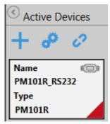
The power meter is now controlled via RS232 operation via the DE-9 or DA-15 port. The status is shown in the field Active Devices next to the device name.
