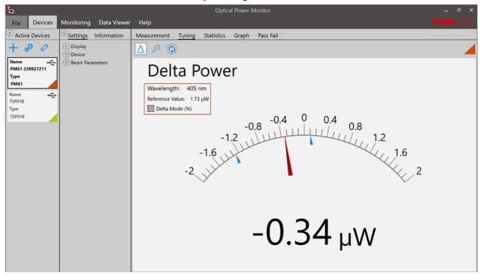
View the "Delta Mode" in % by selecting the check-box: "Delta Mode" (%) in the higher left display.
