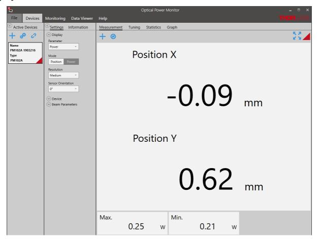
When a Thorlabs Thermal Position Sensor is connected to a power meter and run via the OPM, the OPM menu for "Devices" gives the option to display either the power signal or the positional signal.
