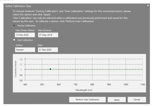
Click "Perform User Calibration" to start a calibration or select and apply a previously saved calibration.
