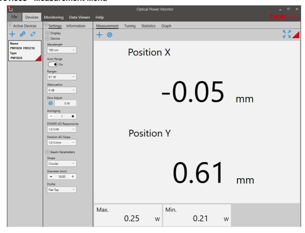
The Measurement interface displays the X and Y - position values and other values selected via the + icon. Options are shown below.
