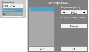
Several responsivities can be added to a list. This way, the correct responsivity can be quickly selected when using different wavelengths.
