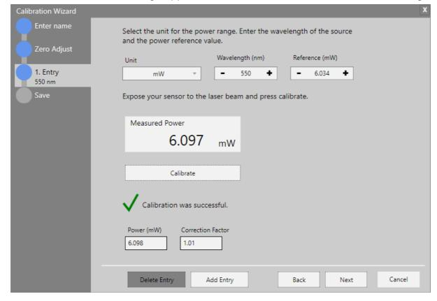
Click "NEXT" to write the calibration data in the internal memory of the power meter and save the results as a .pdf file on the PC by clicking "Write data and save protocol".
