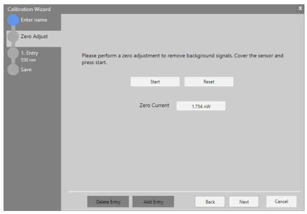
The background is measured. This can be repeated. When the background measurement is finished, click "NEXT" to proceed to the calibration.
