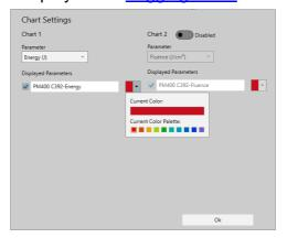
The **Logging Chart** displays the pulse energy values in a continuous line. Please adjust the saving interval according to the interval between the laser pulses in your setup to avoid data points without signal. For pulse intervals shorter than the saving interval, the displayed value is the last value sent by the power meter. For higher resolution measurements, please use the <u>Graph</u> mode.
