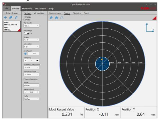
Use the button  $\bigcirc$  to trace the position over time and the icon  $\bigcirc$  to refresh the trace.
