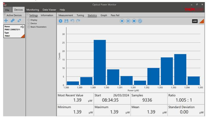
The chart displays the distribution of counts [%] for the parameter selected in <u>Settings</u>. This parameter can be changed during the active measurement. The OPM starts a new data acquisition for statistical analysis when the parameter or monitored device were changed.
