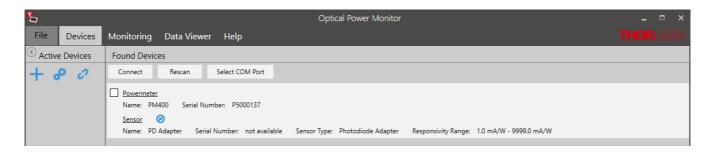
The custom sensor type can be changed under **Settings** in the **Active Devices** panel to either "Photodiode Adapter", "Thermopile Adapter", "Pyro Adapter", or "Four Quadrant" sensor for thermal position sensors.
