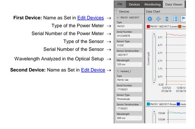
Go to the **Data Chart** and use the <u>Tool Bar</u> to configure the display of devices and parameters.
