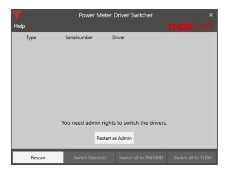
Use the **Menu Bar** at the bottom, to **Rescan** and see all attached devices. The table lists the **Type** of instrument, its **Serial Number** and the currently installed **Driver**.
