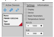
**R25** ( $\Omega$ ): Resistance at 25 °C in Ohm [ $\Omega$ ]
