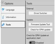
This interface leads you to the driver switcher to change the power meter driver from the former PM100D.dll to the newer TL.dll. While the PM100D.dll supports older software, generated with the older driver, the TL.dll supports all functions of all Thorlabs power meters. Visit the section <a href="Instrument Driver for Thorlabs Power Meters">Instrument Driver for Thorlabs Power Meters</a> for more details.
